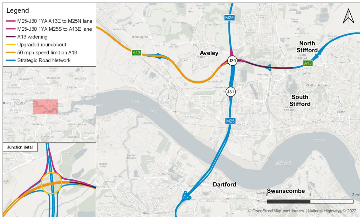
Figure 1 M25 junction 30 location
